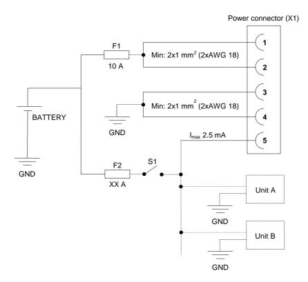
By connecting the power supply according to the illustration above, the device will automatically start when the main switch or turnkey is turned on, and shut down when the switch or turnkey is turned off. While the main switch is in the ON position, the computer can also be turned off and on with the On/Off-button.
